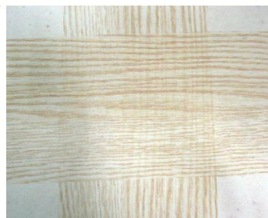
Two stripes of film with normal carrier ( L ) have been superimposed on one another and applied on a white coating: decorations are partially overlapped
