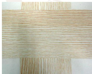
Two stripes of film with L3 carrier: the inks of the upper one (vertical) have been totally blocked by the lower one
