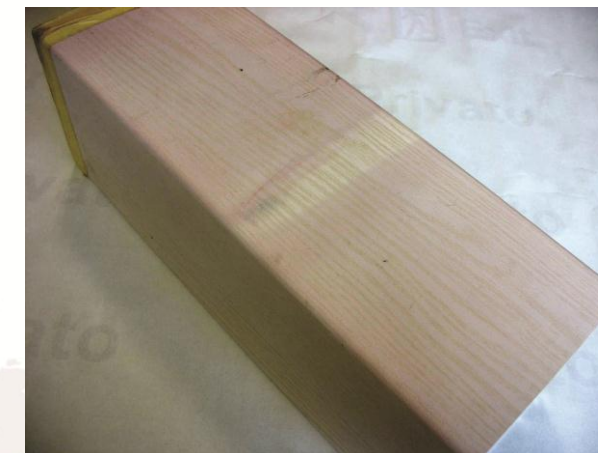
Profile stained by sublimatic inks coming from previous production cycles, passed through the normal carrier L
