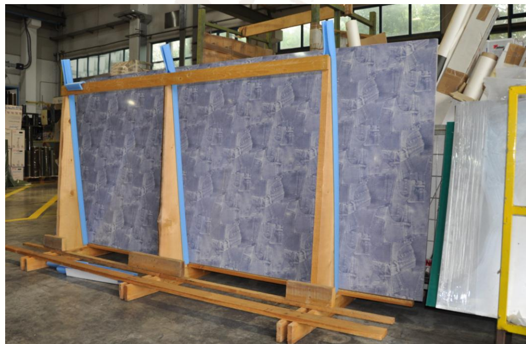
Large flat surface, decorated with heat-transfer matt film 6006/13 M
