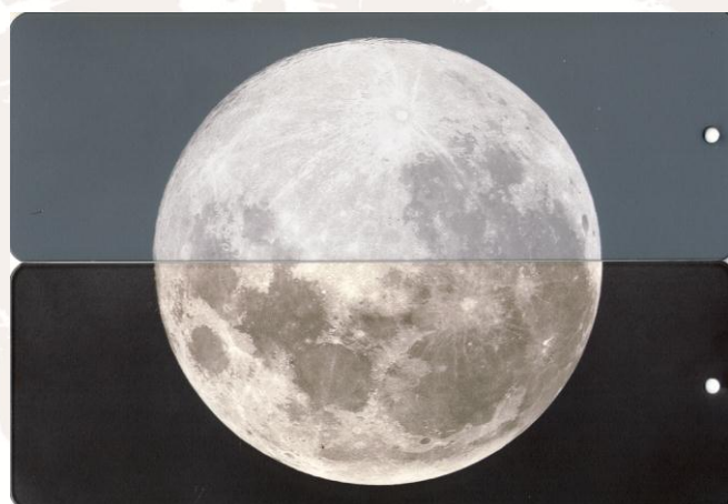
A picture of the moon, heat-transferred on single coat DS 434 (upper panel) and on double coat PE411 + DS 407 (lower)
